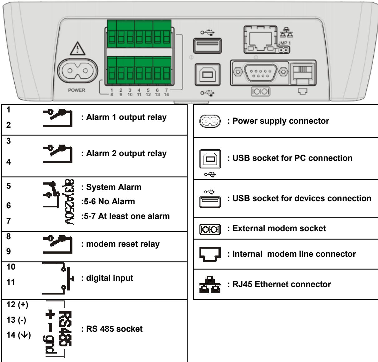
**WARNING:** the relay 'reset modem' is excited to reset, under conditions of disuse every two minutes and before each use (to fax, to dial-up, etc..).
